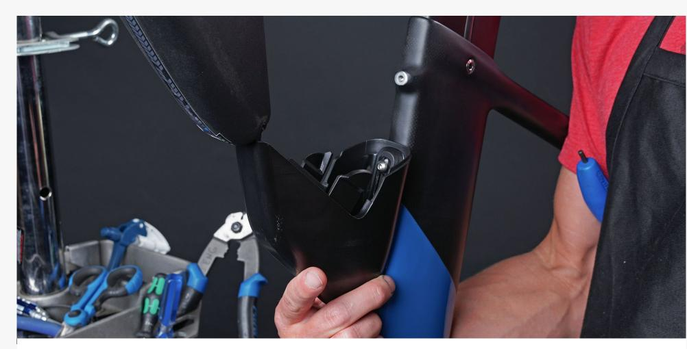
**Step 2:** Install the lower screw. Turn 3 or 4 revolutions.
