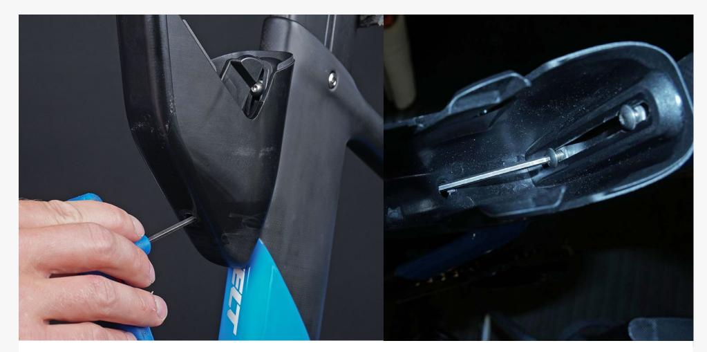
**Step 4:** Tighten the lower screw by inserting a ball-end Hex wrench through the hole on the bottom of the box. Tighten to 4Nm.
